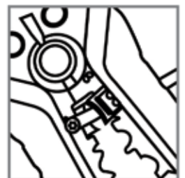
Cut 10-30 AWG (0.05-6mm 2 )
